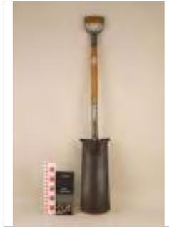
**1973 - 464 Cast Steel Tile Drain Spade**
