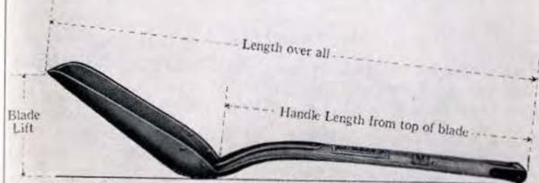
Illustration of side view of Scoop showing dimensions of Length over all, Handle Length from top of blade and Blade Lift
